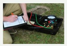
Cross-contamination is the leading cause of waterborne disease. This occurs whenever the water contacts anything that is contaminated or objectionable. Wherever crossconnections can occur is known as a cross-connection. As the water supplier, the city is mandated by State of Oregon drinking water rules (OAR 333-061-0020, 0070 through 0074) to eliminate or control all actual and potential cross-connections.
