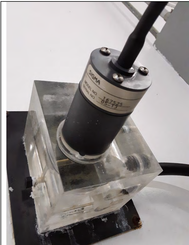
RESIDUAL CHLORINE SENSOR
