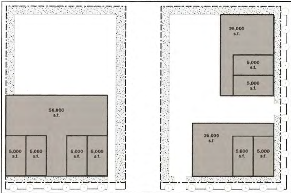
Figure 19.312.4.A Size Limitations for Retail, Service Office, Eating and Drinking Establishments, and Personal Service Uses (Illustrative Example)
