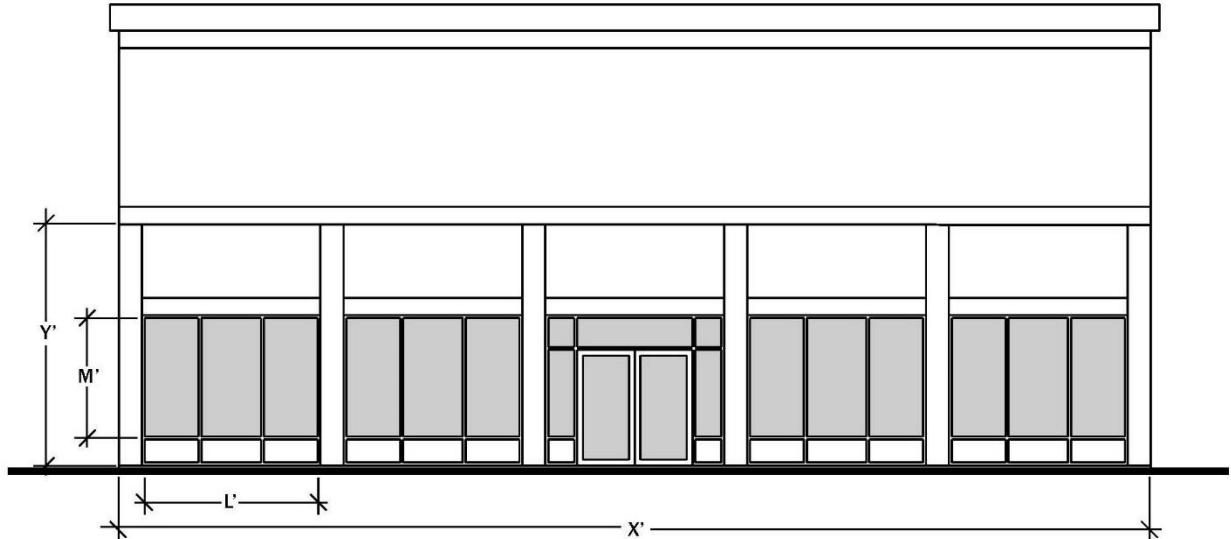
Figure 19.406.5.F.1.a Ground-Floor Windows and Doors
