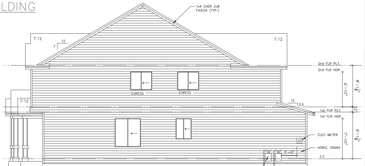
RIGHT ELEVATION 4-PLEX BUILDING SCALE 3/16" = 1'-0"
