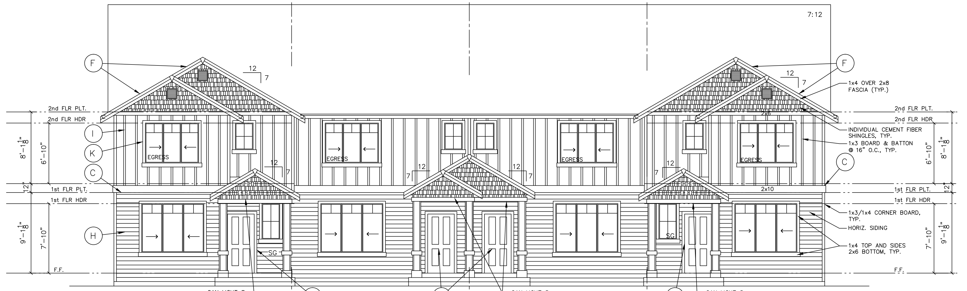
FRONT ELEVATION 4-PLEX BUILDING SCALE 3/16" = 1'-0"
