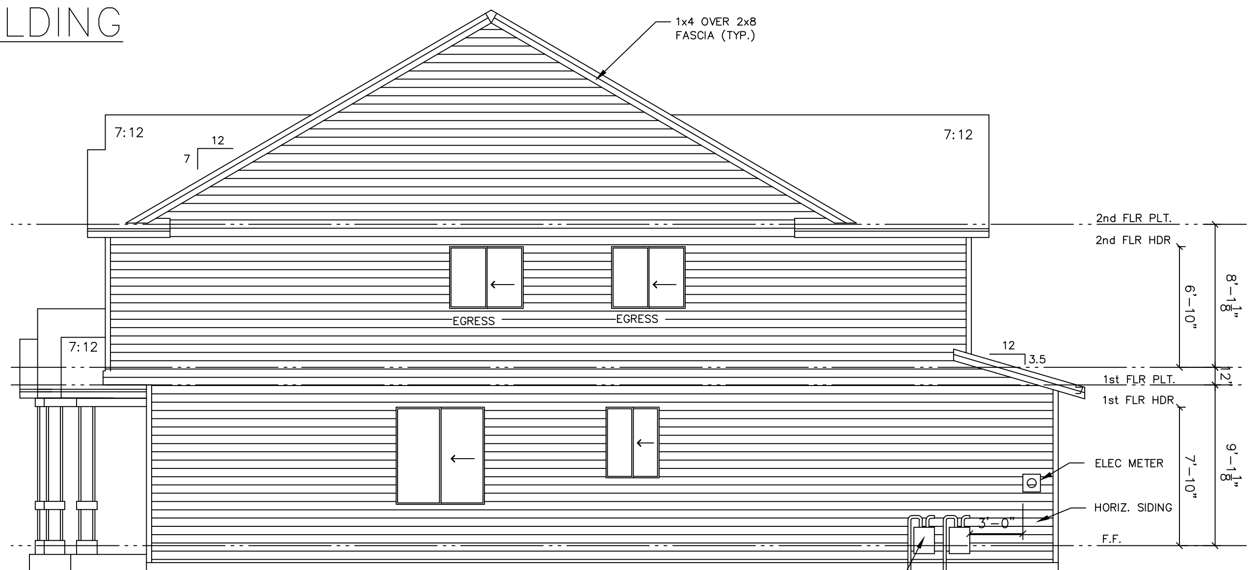
RIGHT ELEVATION 4-PLEX BUILDING SCALE 3/16" = 1'-0"
