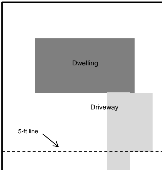
Figure 19.607.1.E.1 Driveway Widening Limitation—Option 1
