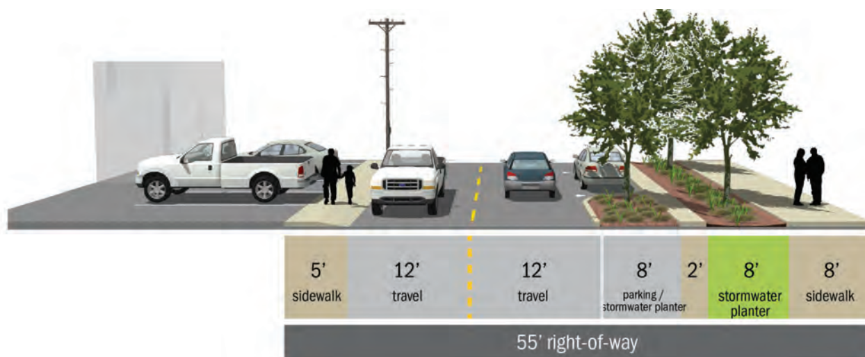
Figure 24. Conceptual Cross-Section for Stubb Street with continuous access (looking east)
