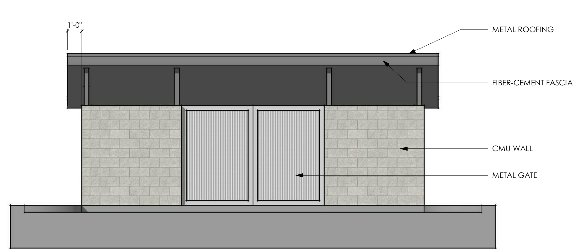
6/ SOUTH ELEVATION - TRASH ENCLOSURE scale: 1/4" = 1'-0"
