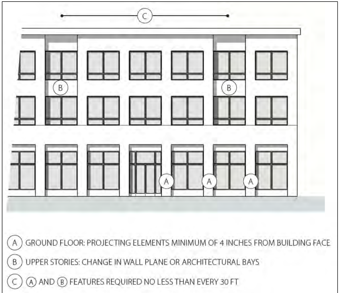
Figure 19.508.4.B.2.b Horizontal Articulation Details
