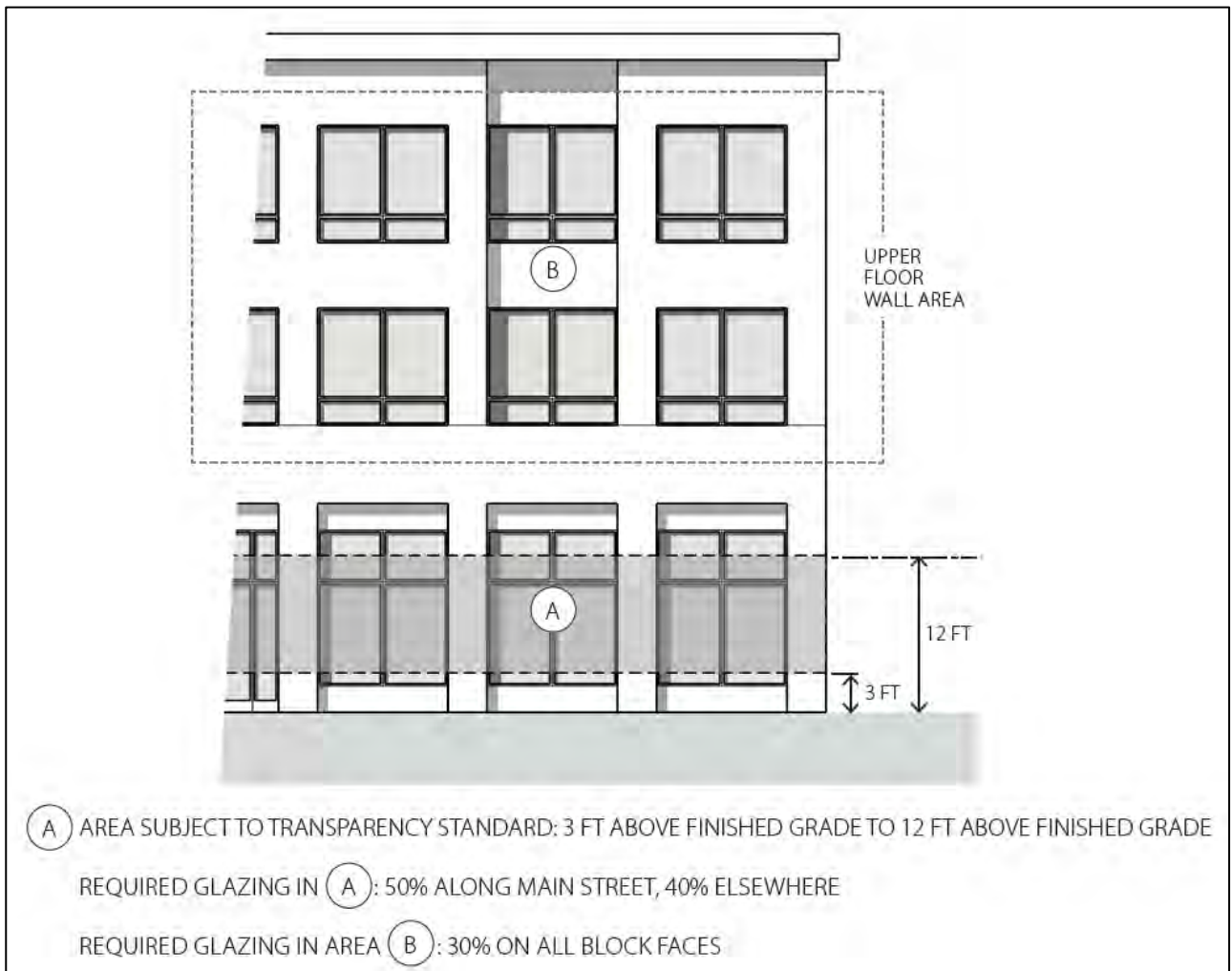
Figure 19.508.4.D.2.b Glazing Standards for Nonresidential and Mixed-Use Buildings
