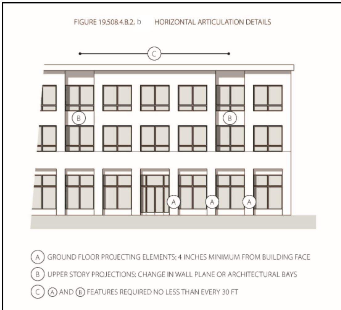
Figure 19.508.4.B.2.b Horizontal Articulation Details
