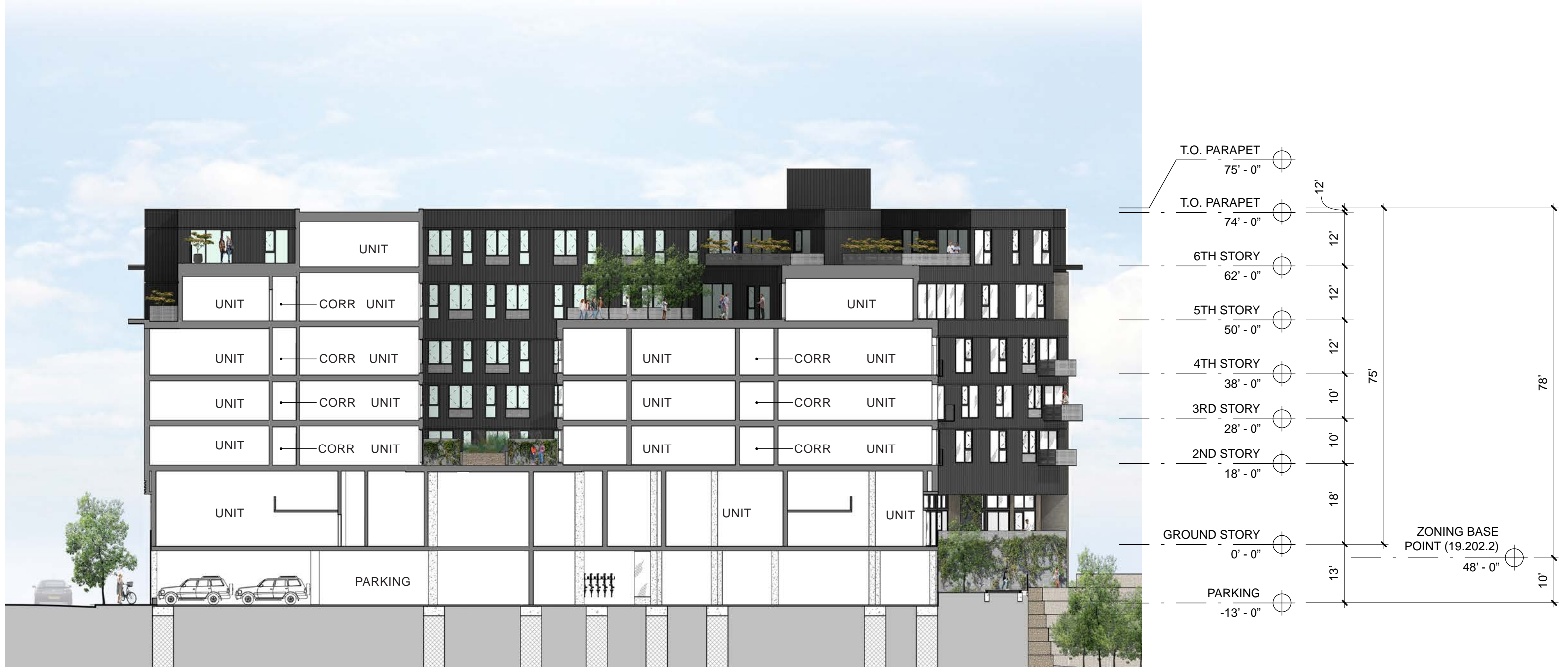
1. BUILDING SECTION SCALE = 3/32"=1'-0"
