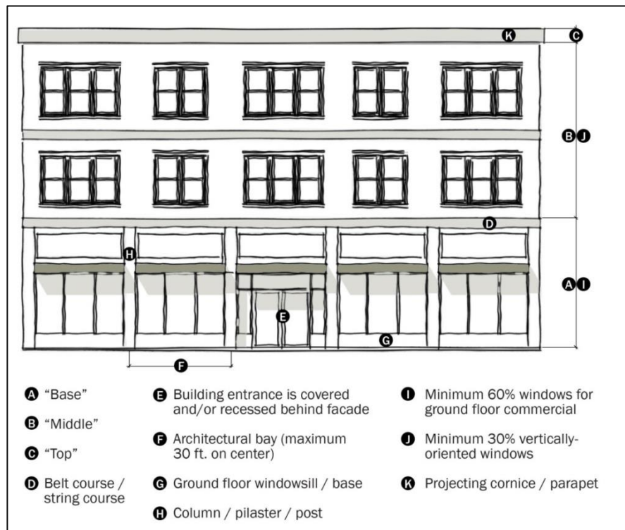
Figure 8. Minimum window and door requirements
