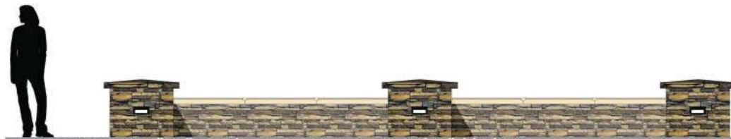
Stone Veneer Seatwall & Pilaster w/ Precast Concrete Caps & Recessed Wall Light Fixture
