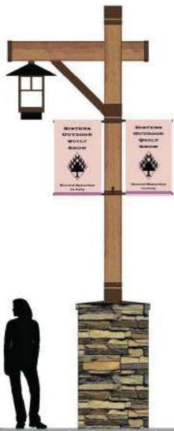
Pedestrian Light Pole w/ Pilaster 'A' (Gateway)
