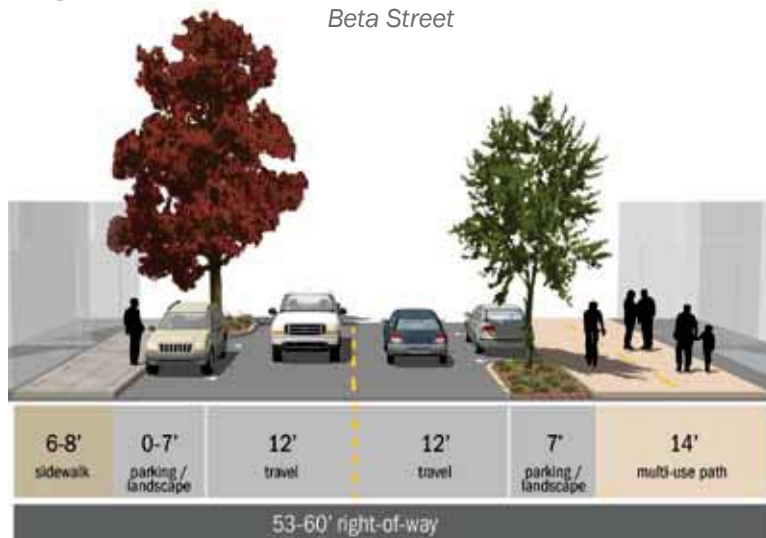
Figure ES-5. Conceptual Cross-Section for Main Street North of Beta Street
