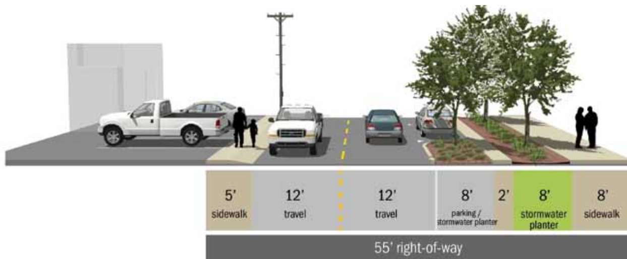
Figure A-11. Conceptual Cross-Section for Stubb Street with continuous access (looking east)
