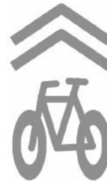
Bicycle Pavement Markings
