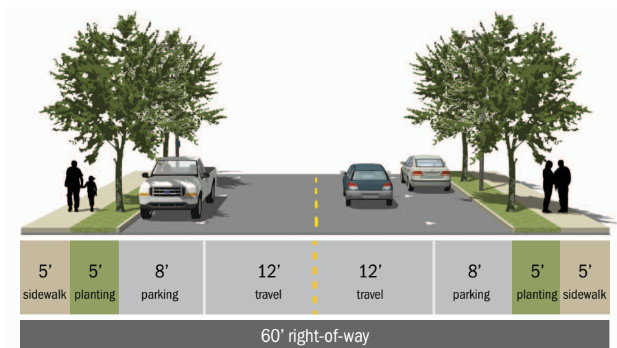
Figure A-11. Proposed Conceptual Cross-Section for Local Streets with a 60' right of way
