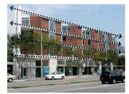
**d.** Datum. Horizontal and linear elements on the facade of the building serve to unify the building. Architectural datums are typically a line or a plane. Examples of datums include projected windowsills and headers, building materials such as a soldier brick course and roof forms. More subtle examples of datums include window mullions, ground floor awnings and a belt course or sign band.
