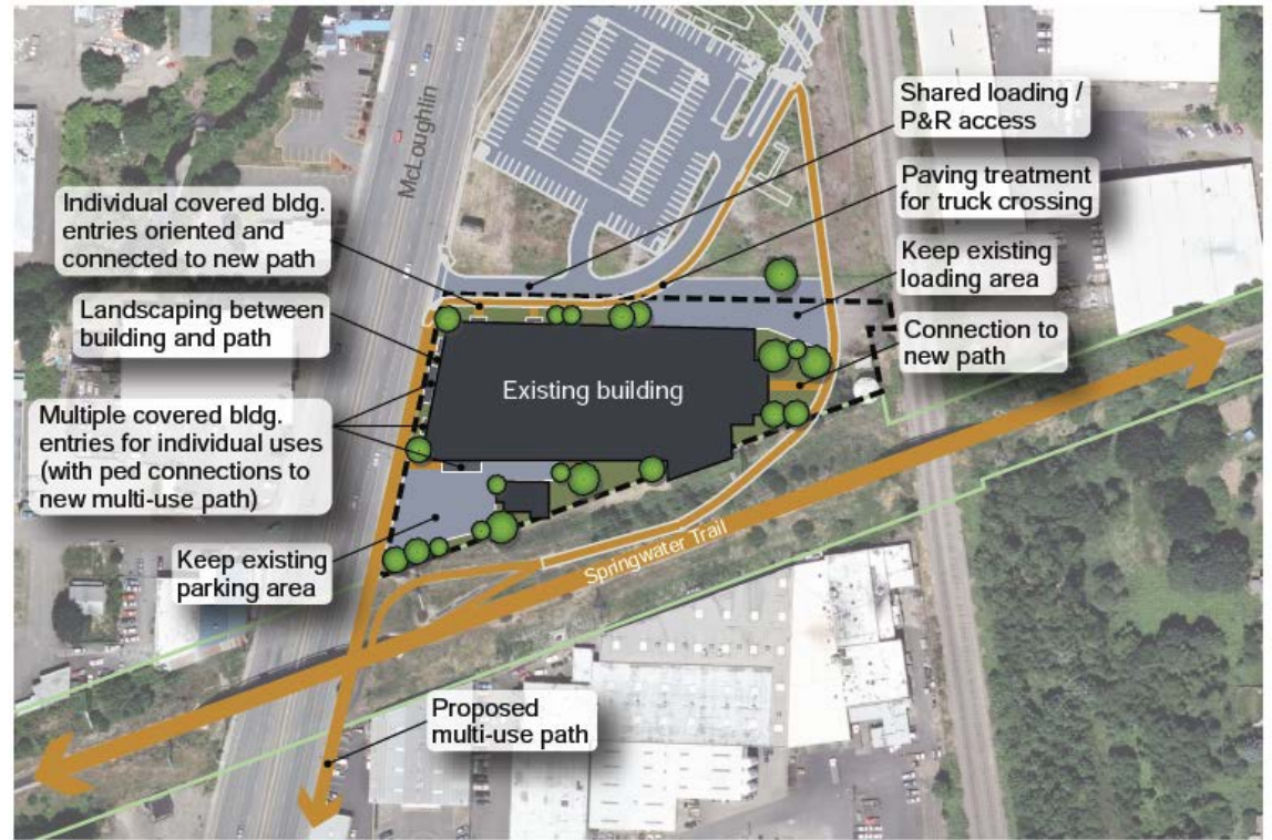
Figure 5. Conceptual Site Plan for Redevelopment of Opportunity Site A under all three scenarios
