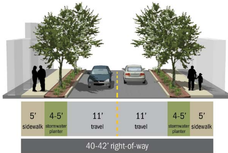
Figure A-9. Proposed Conceptual Cross-Section for Local Streets with a 40' right of way
