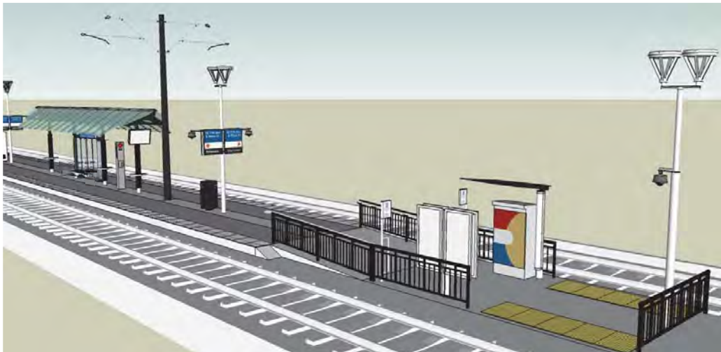
Station-specific Shelter and TVM Shelter With Other Platform Amenities
