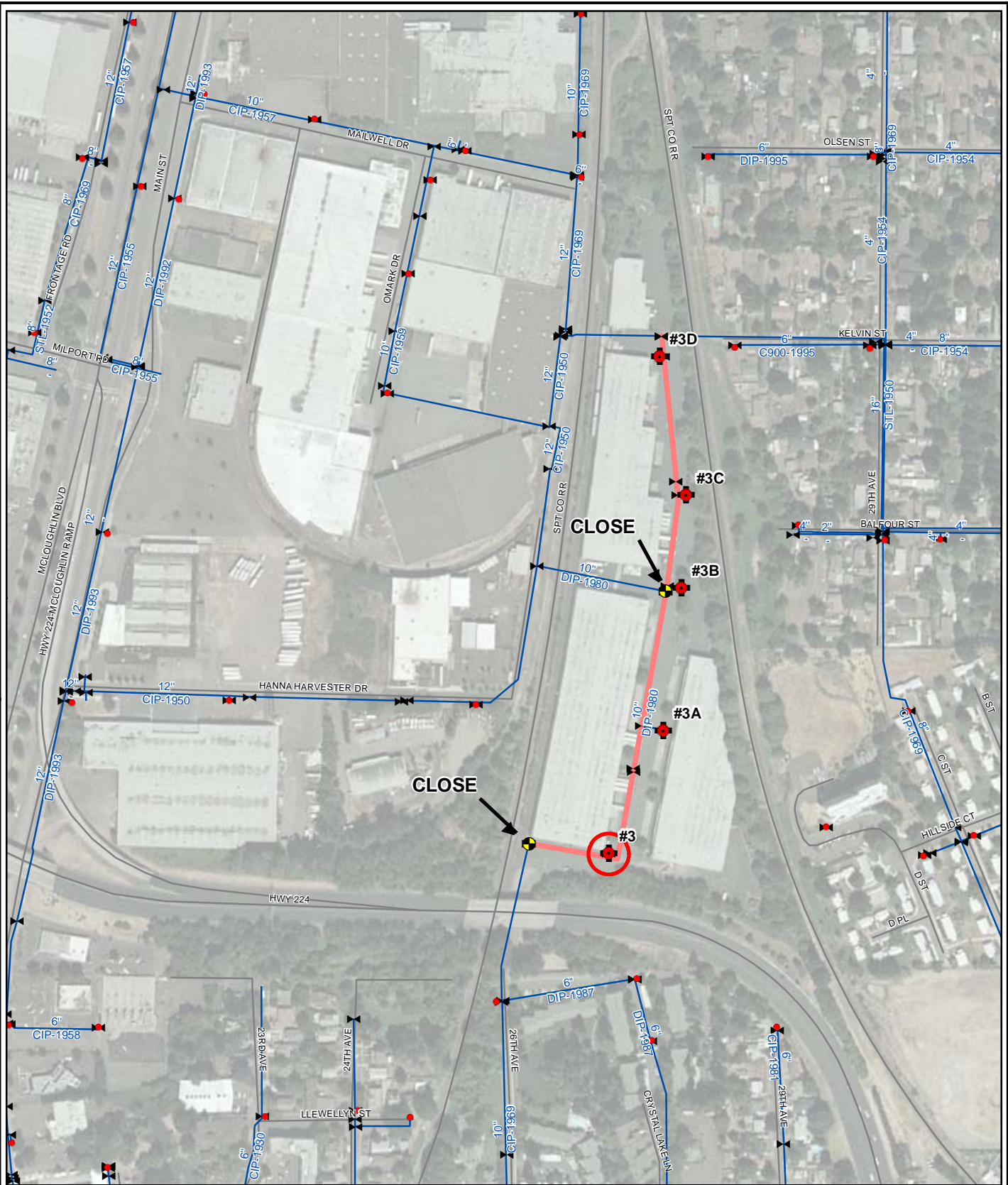
FIGURE A-3 City of Milwaukee Water System Master Plan TEST #3 (10" DIP 1980)
