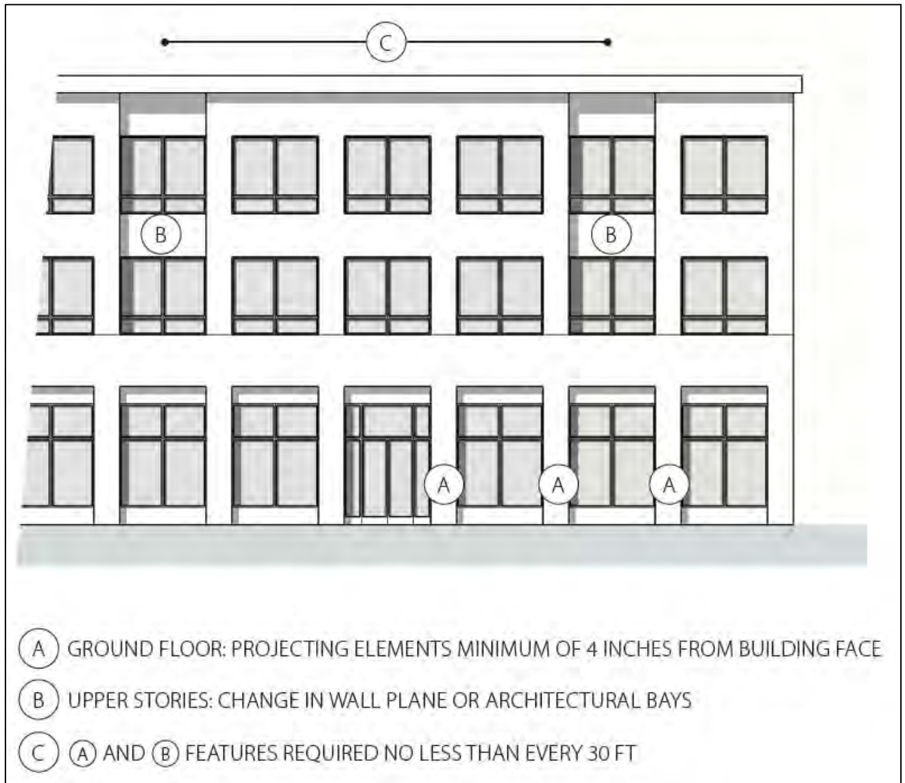
Figure 19.508.4.B.2.b Horizontal Articulation Details
