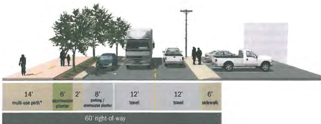
Figure 23. Conceptual Cross-Section for Mailwell Drive with continuous access (looking east)
