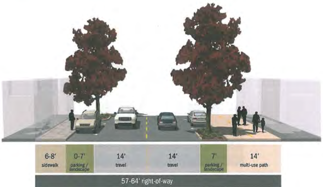
Figure 16. Conceptual Cross-Section for Main Street – North of Beta Street within existing right-of-way (looking north)
