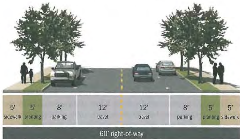
Figure 21. Proposed Conceptual Cross-Section for Local Streets with a 60' right of way
