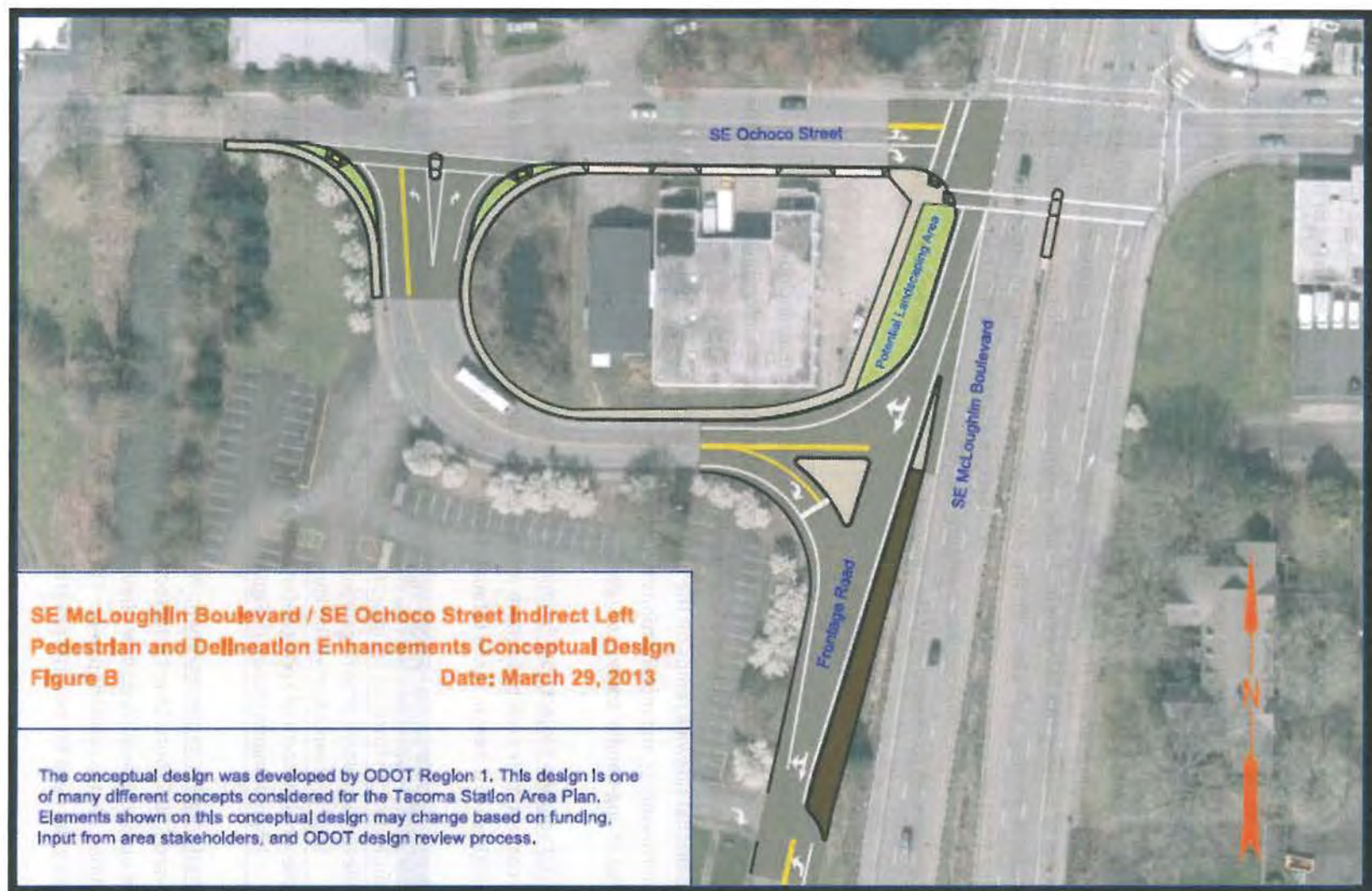
Figure B. Indirect Left Pedestrian and Delineation Enhancements Conceptual Design
