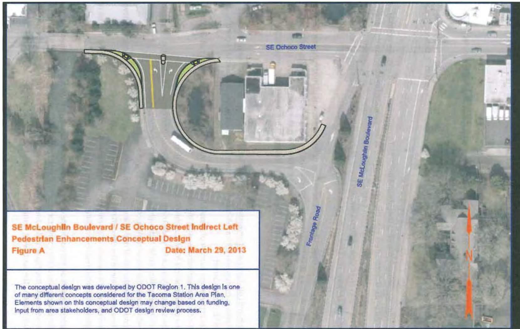
Figure A: Indirect Left Pedestrian Enhancements Conceptual Designs
