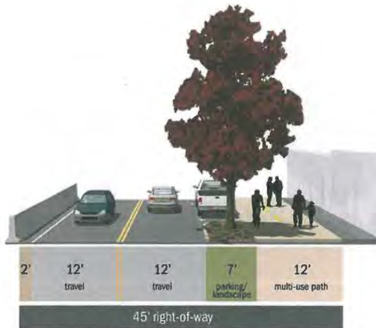
Figure 15. Conceptual Cross-Section for Main Street – Milport Road to Beta Street within existing right-of-way (looking north)
