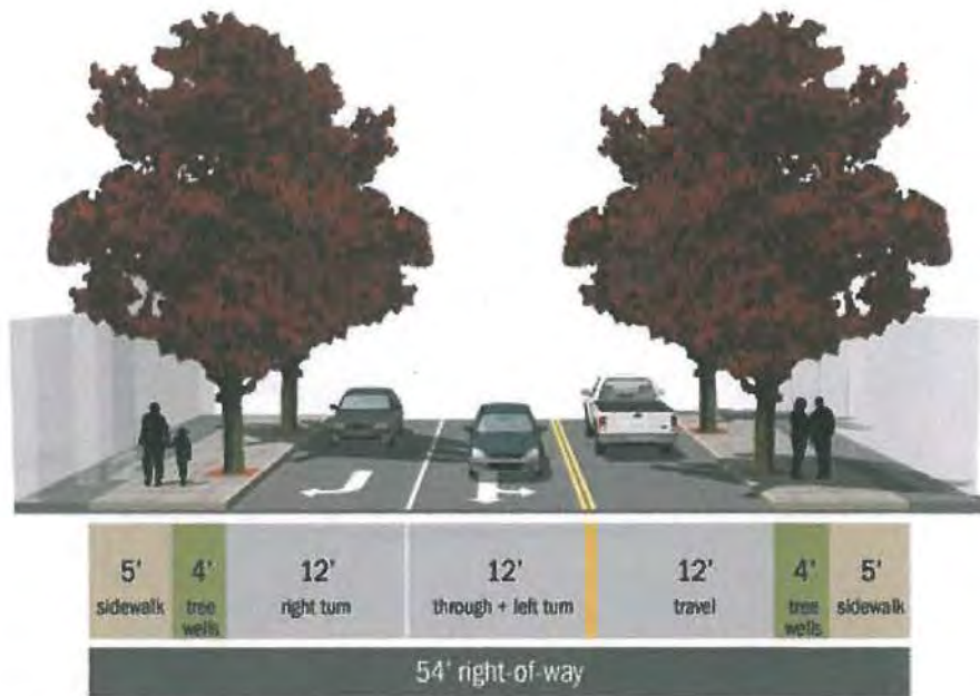
Figure 17. Conceptual Cross-Section for Ochoco Street – West of Main Street within existing right-of-way (looking east)
