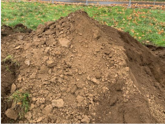
11/1/21 Parcel 1 NE corner soil test pit showing high organic content.
