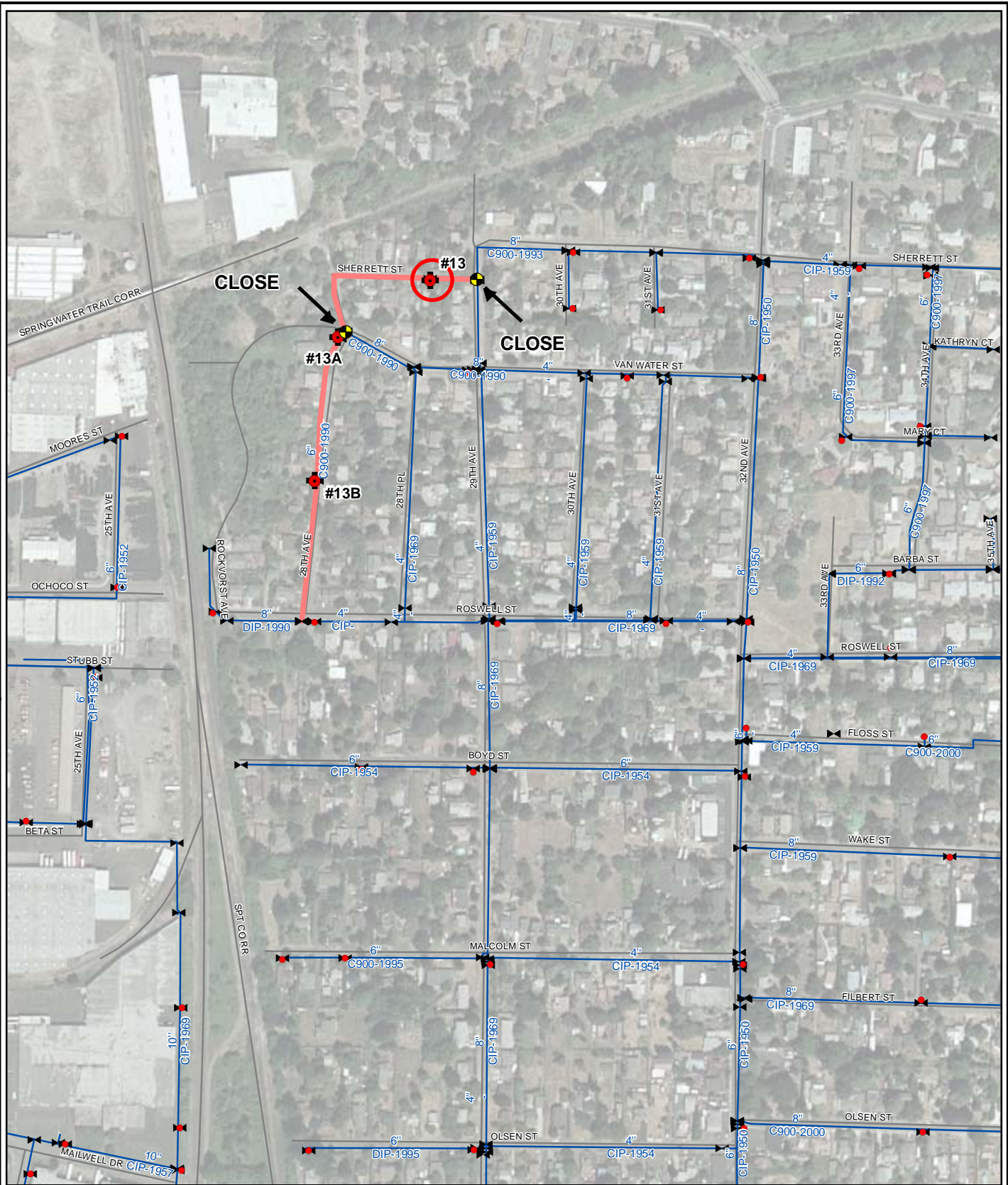
FIGURE A-13 City of Milwaukee Water System Master Plan TEST #13 (6" PVC 1993)
