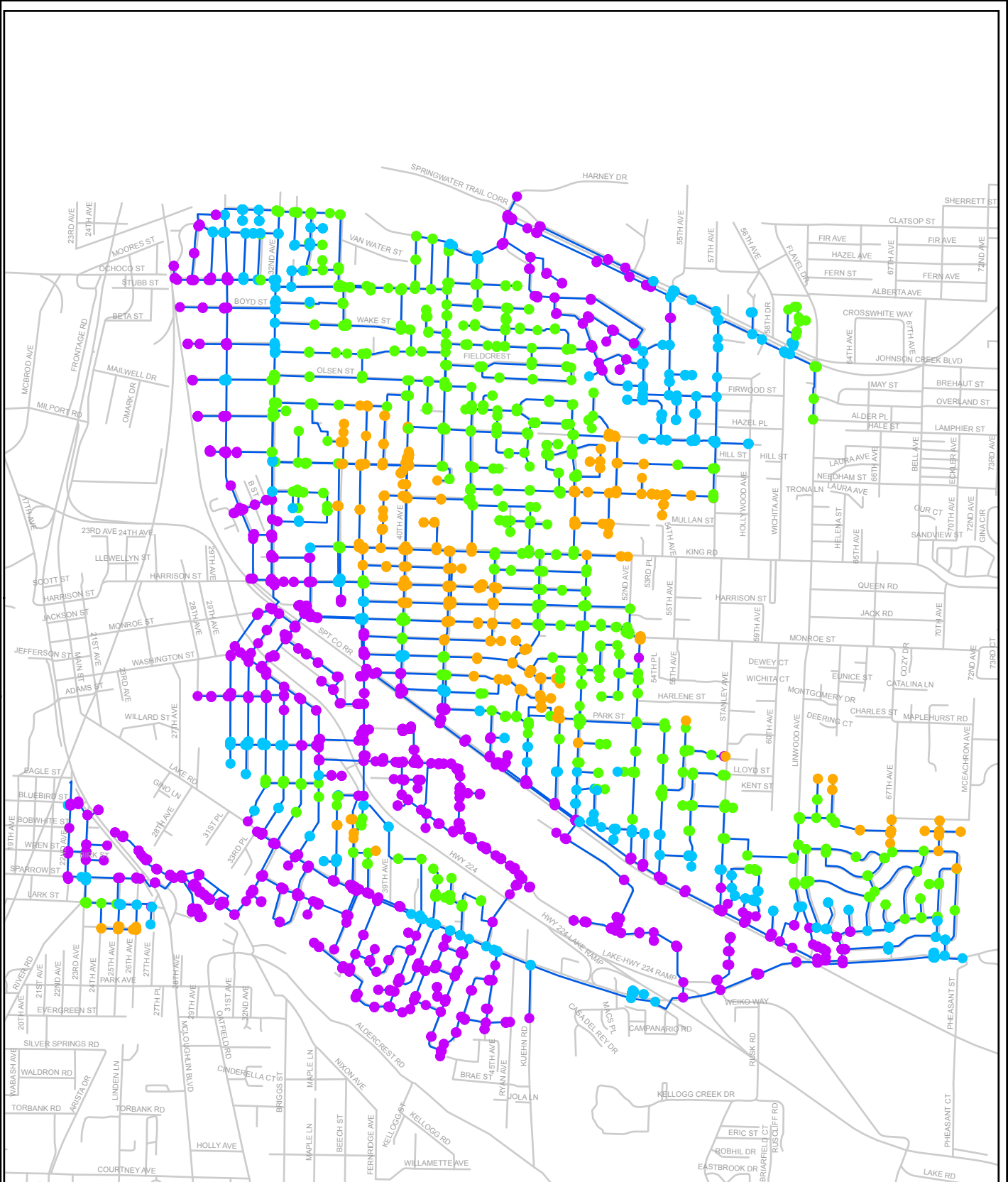
FIGURE 8-7 City of Milwaukee 2010 Water System Master Plan PRESSURE ZONE 2 PEAK HOUR ANALYSIS BUILDOUT SYSTEM
