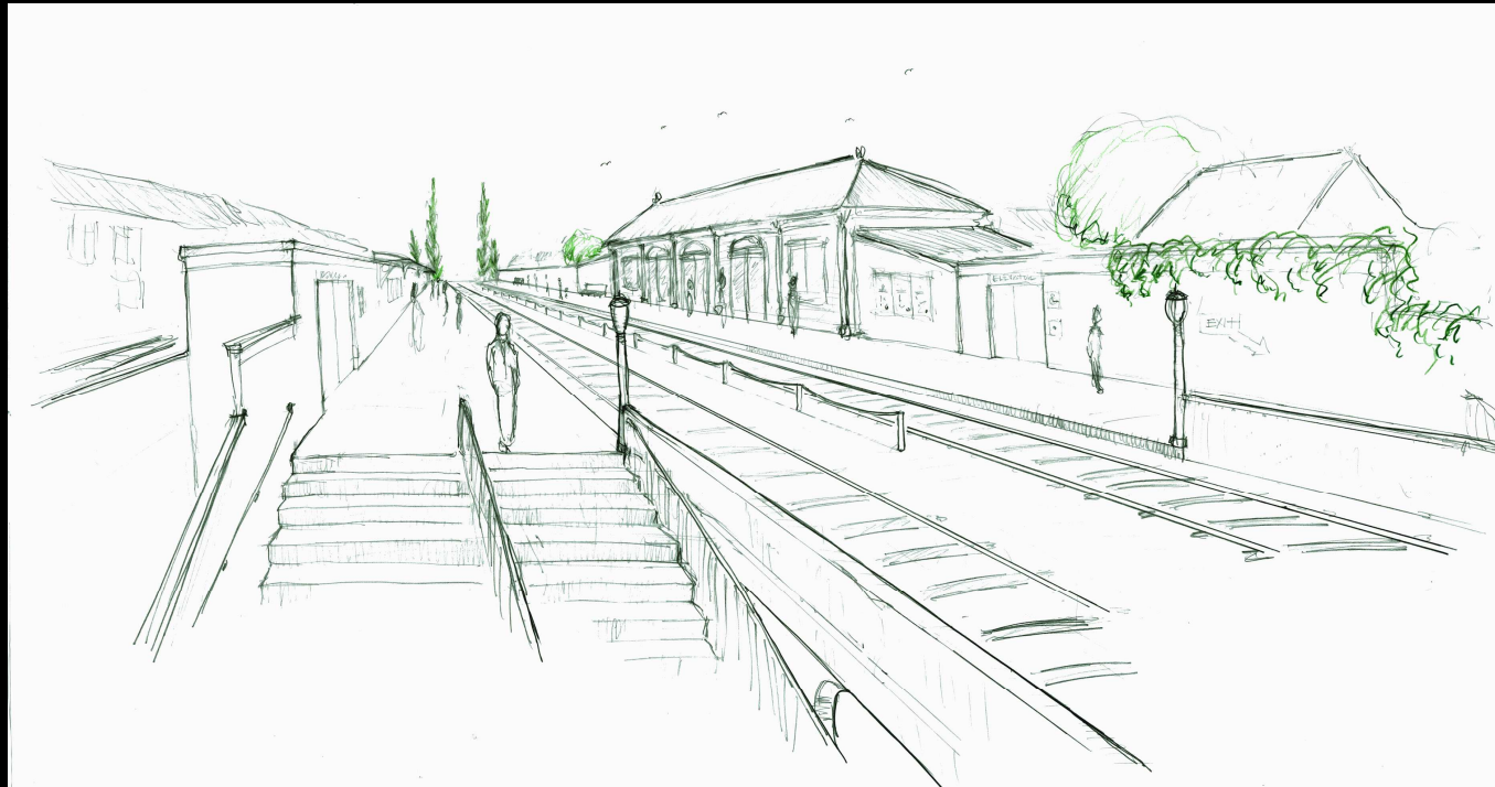
Rough sketch of platform area looking north, showing split platform, beginning of narrow bridge, steps to Lake Road, and waiting building on northbound platform
