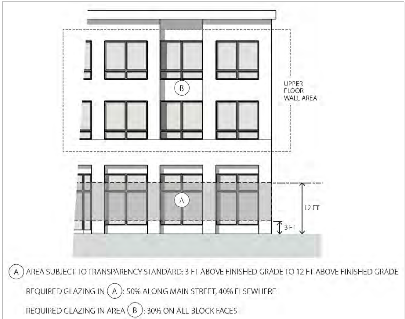
Figure 19.508.4.D.2.b Glazing Standards for Nonresidential and Mixed-Use Buildings
