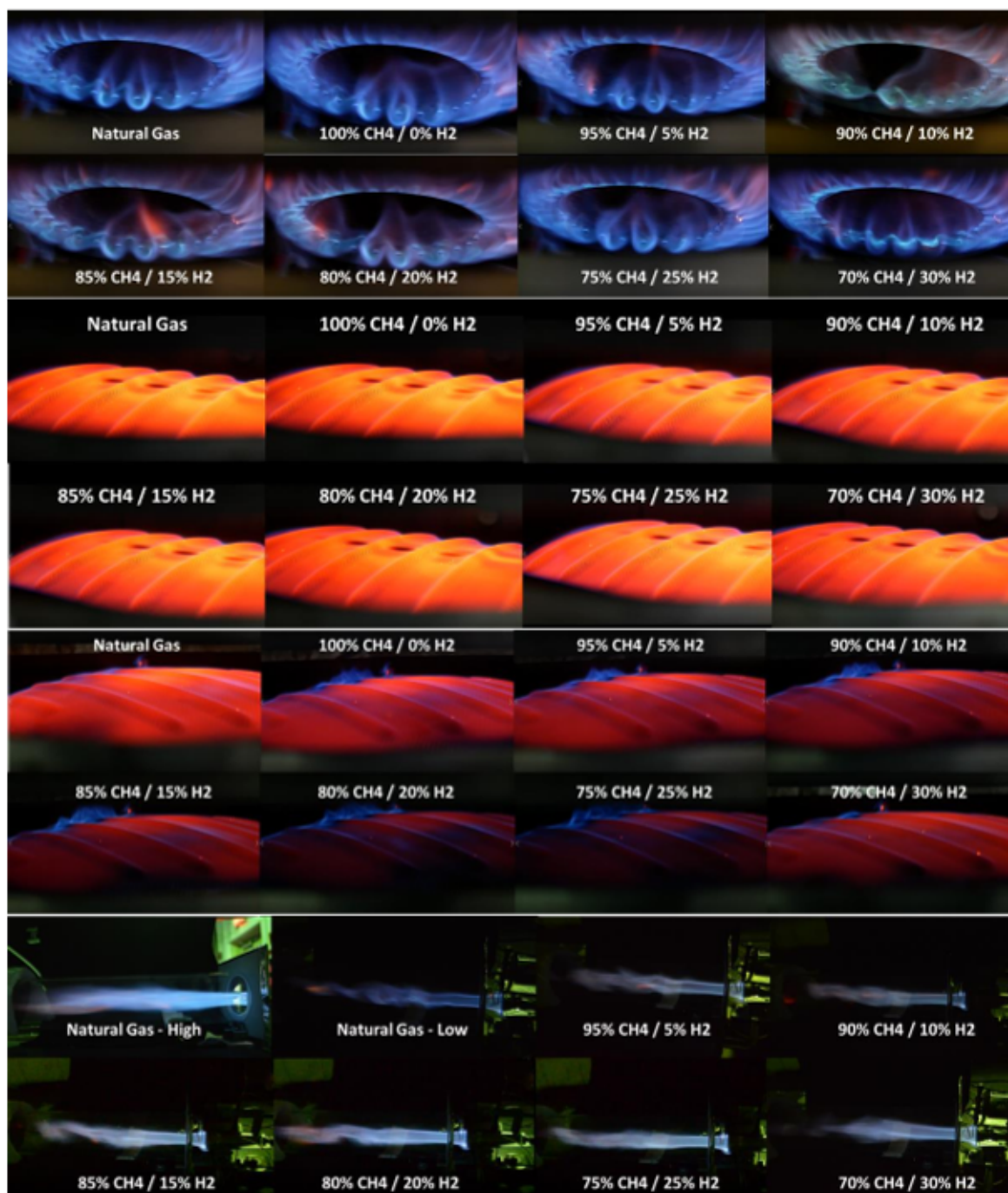
Figure 8. Still images of water heater and furnace burners during simulator testing.
