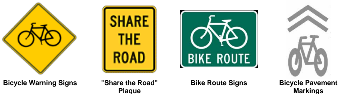
Figure 6-1 Bicycle Signs and Markings
