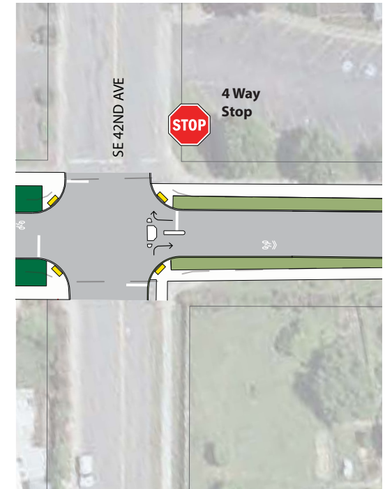
Diverter at 42nd Avenue and Monroe
