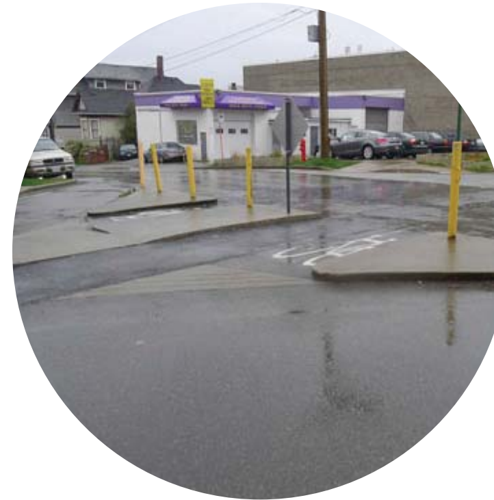
Example of a right-in/right out diverter
