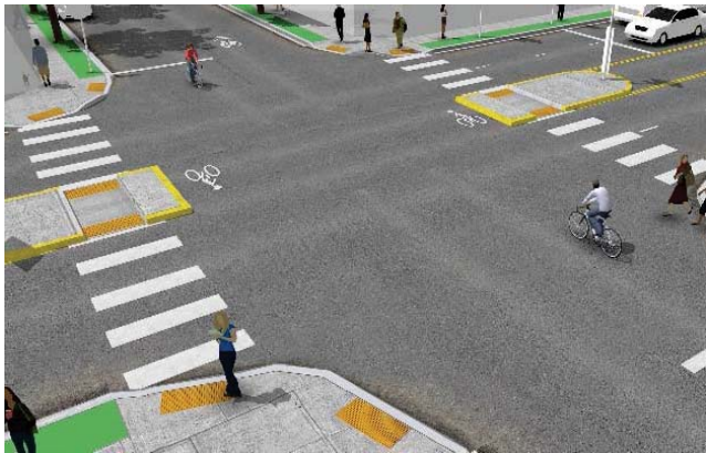
Example of intersection with median refuge islands
