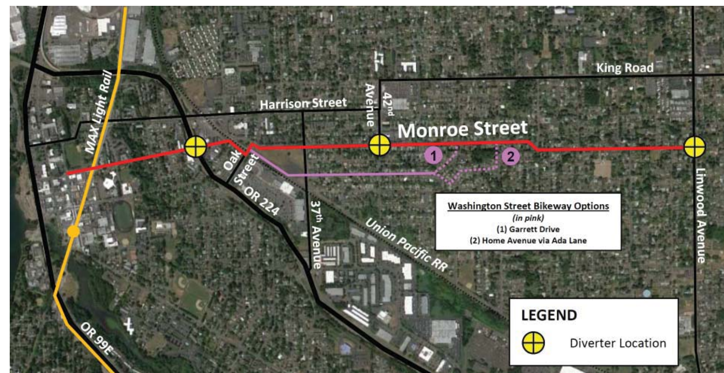
Red line is Monroe only alignment; pink line shows possible options for the Monroe-Washington route
