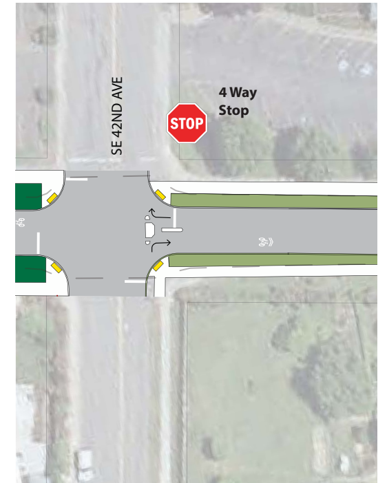
Diverter at 42nd Avenue and Monroe
