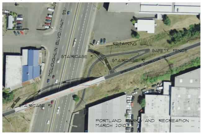
Figure 2. Planned Improvements from Springwater Corridor to Light Rail Station
