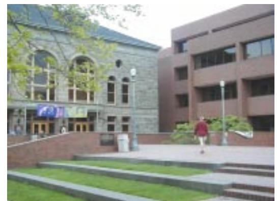
Not Recommended: New building makes no acknowledgement of the historic building's facade configuration or materials (Seattle, WA)
